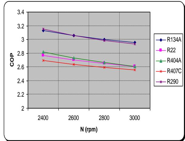
Figure 8: Variation of first law efficiency in terms of coefficient of performance (COP) with speed of compressor of different ecofriendly refrigerants
